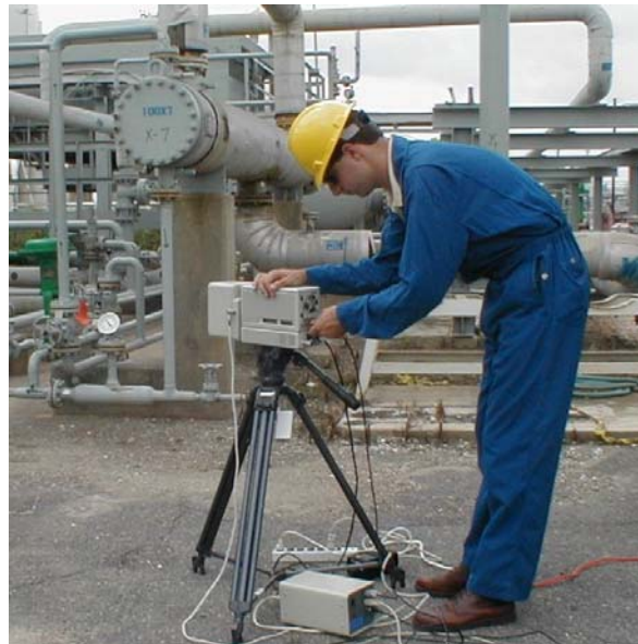
Figure 4. IMSS on Radiance 1 infrared Camera in oil refinery.
